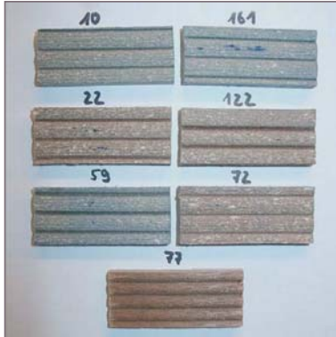
Fig. 3: Selected test specimen after mould fungi test: no vegetation macroscopically detectable
